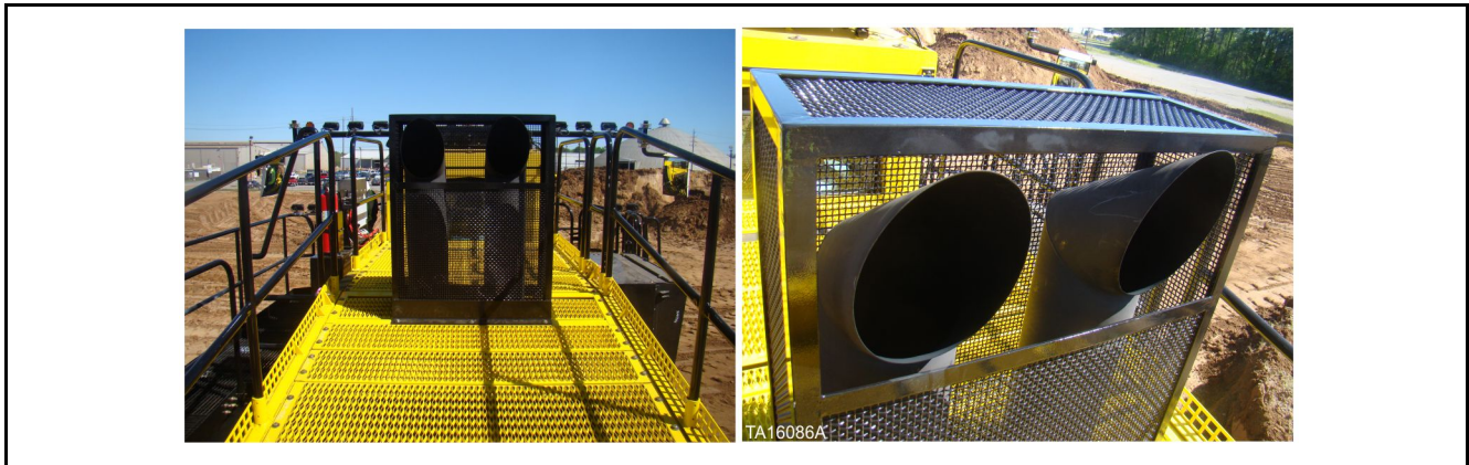
Figure 19. Engine exhaust stacks guard assembly
