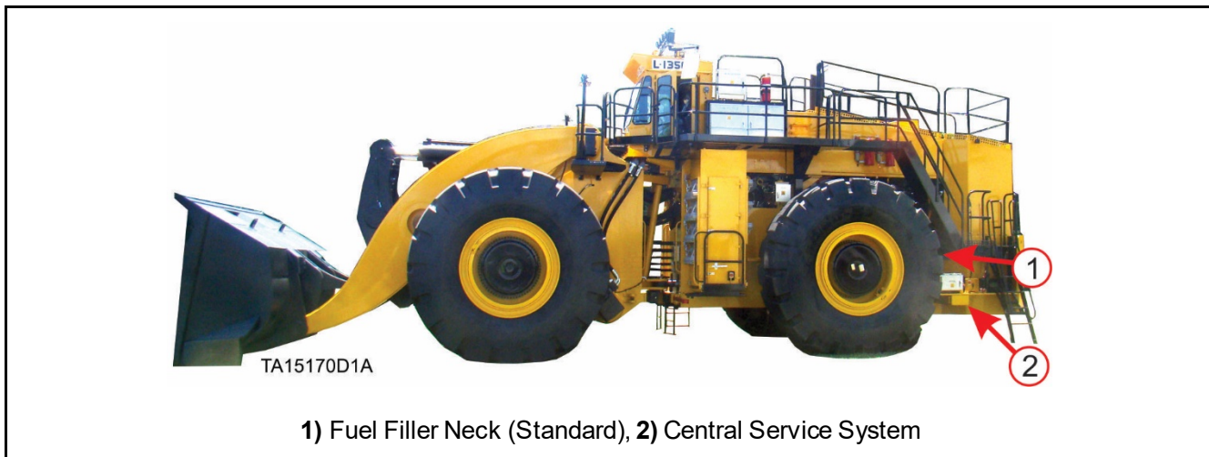
Figure 2. Typical fuel filler location
